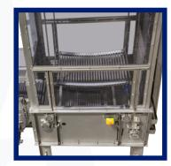
Sanitation was a key design driver, especially for facilities operating under strict food safety protocols. Built entirely from stainless components, the system is fully washdown capable and designed for quick, efficient cleaning. This not only supports regulatory compliance but also minimizes downtime during cleaning and maintenance.
